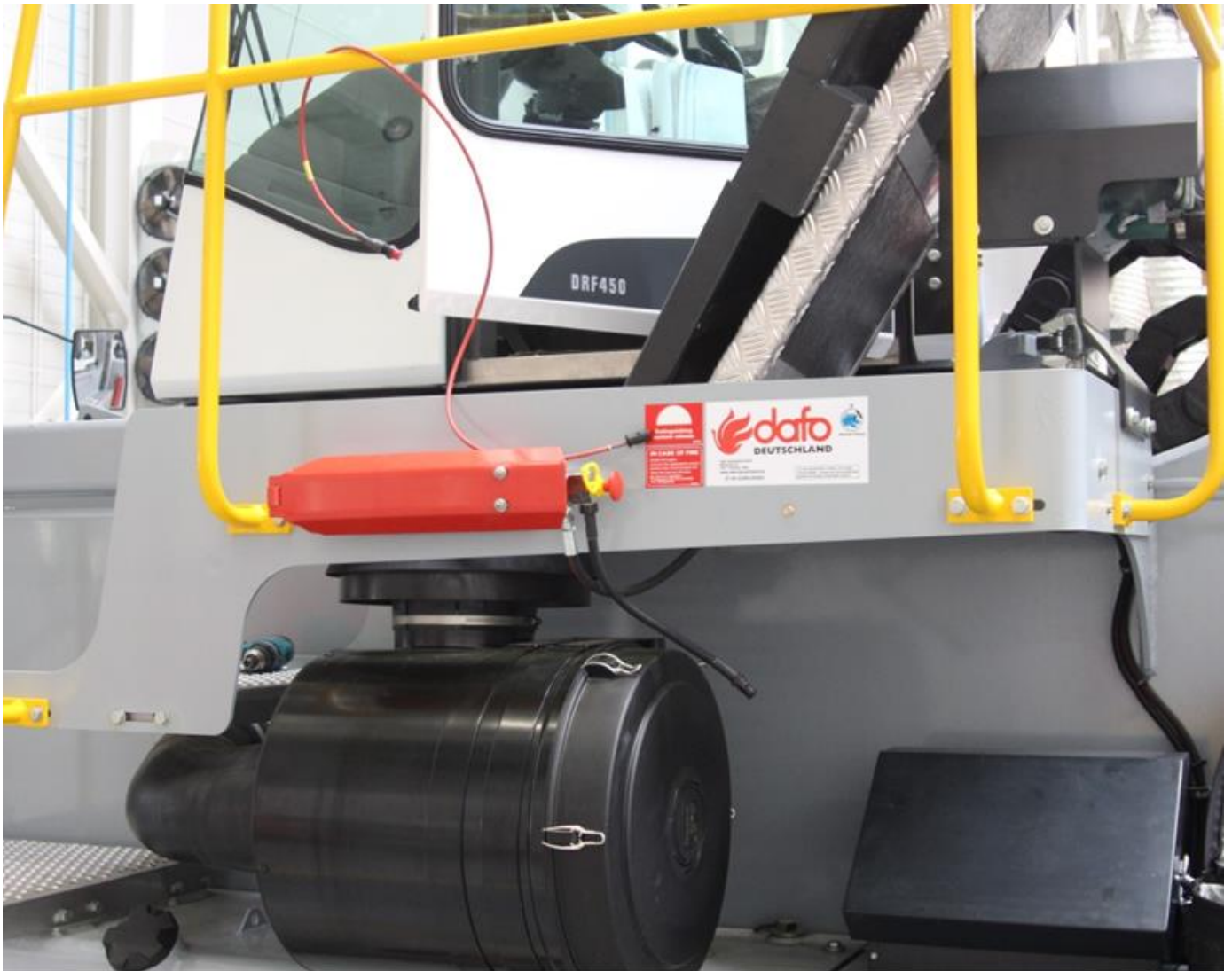
FORREX SV-K 11250 (25 L) installed in Kalmar DRF450 Reachstackers
