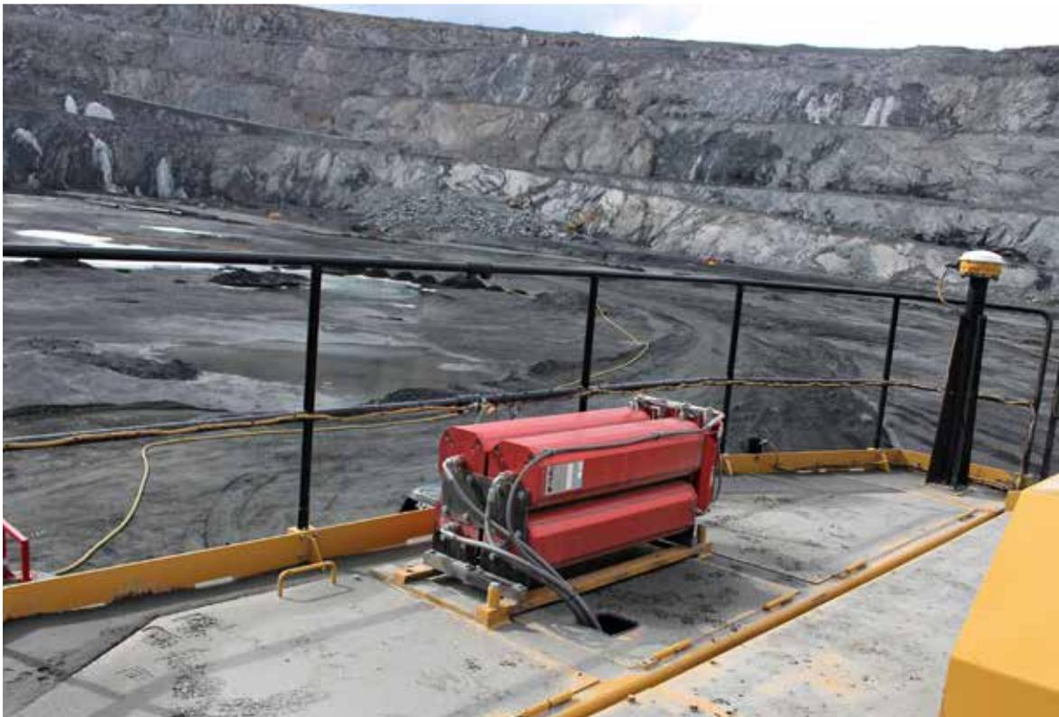
**Suppression:** The distribution network is composed of flexible fire resistance hydraulic hoses, stainless steel pipes with full cone nozzles that will protect all areas or specifically locations with many potential fire hazards such as turbo charger, catalytic converter, pumps, fuel lines, generators, transmission belts, filters and hydraulic package.
