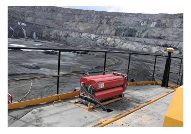
**Suppression:** The distribution network is composed of flexible fire resistance hydraulic hoses, stainless steel pipes with full cone nozzles that will protect all areas or specifically locations with many potential fire hazards such as turbo charger, catalytic converter, pumps, fuel lines, generators, transmission belts, filters and hydraulic package.
