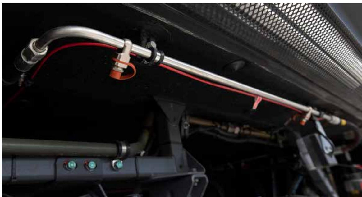
Large heavy-duty mining vehicles have large engine compartments. It is therefore important that the engine compartments are protected with additional suitable detection systems in addition to the linear heat detector which then provides the vehicle maximum fire protection.
